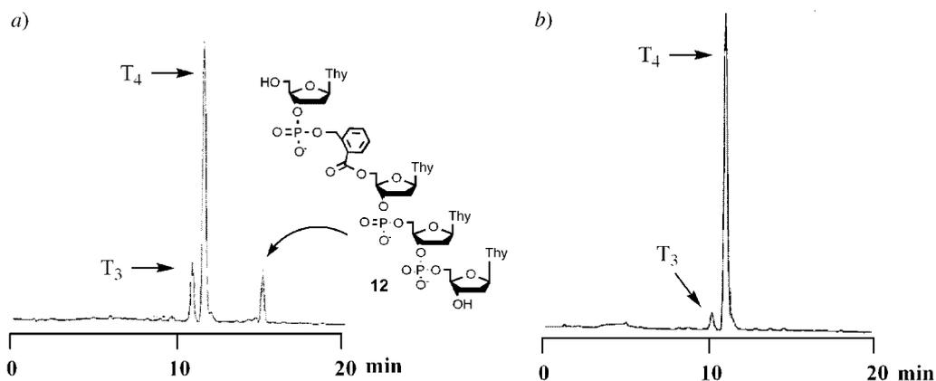
Fig. 1. Reversed-phase HPLC profiles of T<sub>4</sub> synthesized by a combination of conventional (MeO)<sub>2</sub>Triphosphoramidite and MOB-phosphoramidite **11** for a time period of a) 1 min and b) 5 min for Step 3b in Scheme 8, resp.
