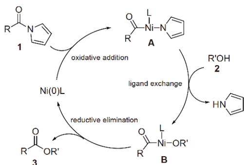
**Scheme 2** A plausible mechanism for the Ni-catalyzed alcoholysis of *N*-acylpyrrole-type tertiary amides (R=aryl; alkyl).
