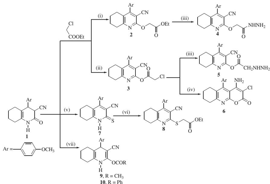
(i) K<sub>2</sub>CO<sub>3</sub>, acetone, reflux for 30h; (ii) K<sub>2</sub>CO<sub>3</sub>, DMF, reflux for 9h; (iii) N<sub>2</sub>H<sub>4</sub>·H<sub>2</sub>O, EtOH reflux for 11h; (iv) 10% alc. KOH reflux for 6h; (v) P<sub>2</sub>S<sub>5</sub>, toluene reflux for 4h; (vi) ClCH<sub>2</sub>COOEt, CH<sub>3</sub>COONa, EtOH, reflux for 4 h; (vii) Ac<sub>2</sub>O, and / or PhCOCl, pyridine, reflux for 5h
