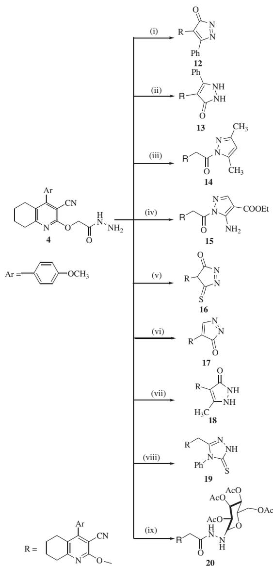
(i) Benzoyl chloride, reflux for 12h; (ii) Benzoic acid, POCl<sub>3</sub>, reflux for 10h; (iii) Acetyl acetone, EtOH, reflux for 17h; (iv) 2-Ethoxymethylene-cyanoacetate, EtOH, reflux for 19h; (v) CS<sub>2</sub>, KOH, EtOH, reflux for 12h; (vi) Formic acid, reflux for ; (vii) Acetic acid, reflux for 12h; (viii) Phenyl isothiocyanate, pyridine, reflux for 9h; (ix)  $\alpha$ -D-Glucose pentaacetate, EtOH, reflux for 35h
