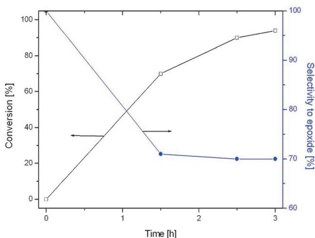
**Figure 1.** Conversion of 4-methylstyrene and selectivity to epoxide as a function of time at 298 K, 14.5 psi oxygen pressure.
