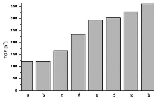
**Figure 3.** Comparison of TOF (h<sup>-1</sup>) of: (a) cyclohexene, (b) styrene, (c) 1-phenyl-1-cyclohexene, (d) 1-methyl-1-cyclohexene, (e) *R*-(+)-limonene, (f) (-)- $\alpha$ -pinene, (g) 4-methylstyrene, and (h)  $\alpha$ -methylstyrene, over LDH hosted Mn-salen catalyst.
