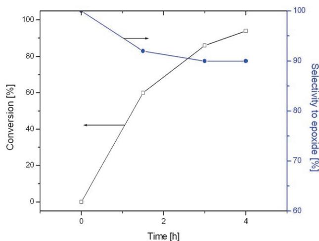
**Figure 2.** Conversion of 1-methyl-1-cyclohexene and selectivity to epoxide as a function of time at 298 K and 14.5 psi oxygen pressure.
