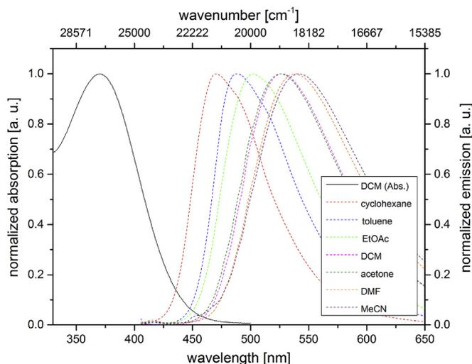
Fig. 4. UV/Vis absorption in dichloromethane (solid line) and emission (dashed lines) spectra in seven solvents of different polarity (recorded at  $T = 293$  K).
