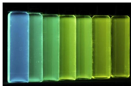
Fig. 3. Fluorescence of **3k** with variable solvent polarity (left to right: cyclohexane, toluene, ethyl acetate, dichloromethane, acetone, *N,N*-dimethyl formamide, acetonitrile;  $\lambda_{\text{exc}} = 365$  nm, hand-held UV lamp).
