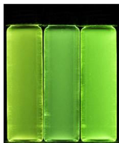
Fig. 1. Fluorescence of phenothiazinyl propiolates **3k–l** (left to right,  $\lambda_{\text{exc}} = 365$  nm, hand-held UV lamp).
