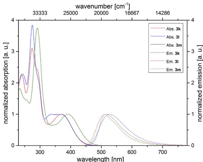
Fig. 2. UV/Vis absorption (solid lines) and emission (dashed lines) spectra of phenothiazinyl propiolates **3k–l**. Recorded in dichloromethane,  $T = 293$  K.
