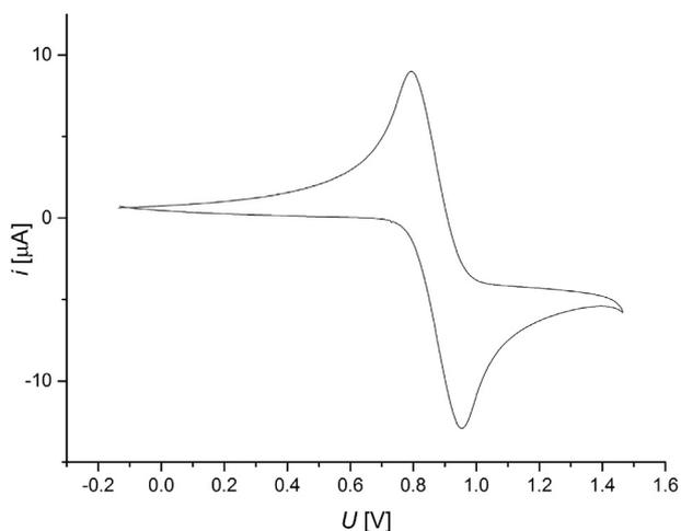
**Fig. 7.** Cyclic voltammogram of **3k** (recorded in dichloromethane,  $T = 293$  K, 0.1 M electrolyte  $[\text{Bu}_4\text{N}][\text{PF}_6]$ , Pt working electrode, Pt counter electrode, Ag/AgCl reference electrode).
