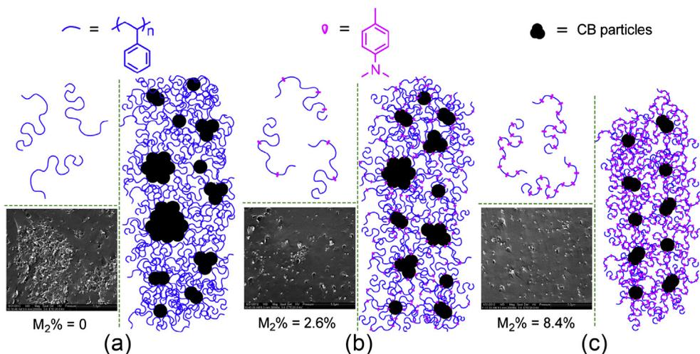
**Fig. 6.** Representation of the structure models of CB-based polymer composites as a function of the geminal dimethylamino group content  $M_2\%$ : (a) large CB agglomerates coexisting with aggregates, (b) small and less CB agglomerates along with aggregates, and (c) CB aggregates.
