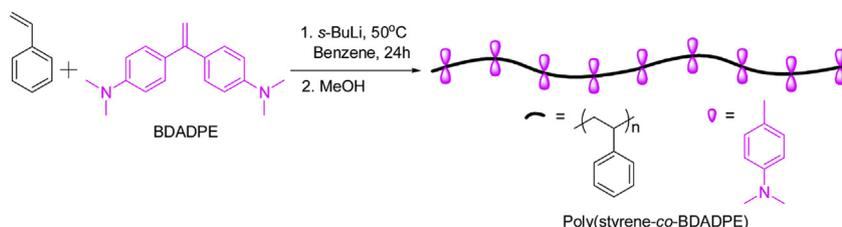
Scheme 1. Synthesis of in-chain multi-functionalized polystyrene using BDADPE as comonomer.
