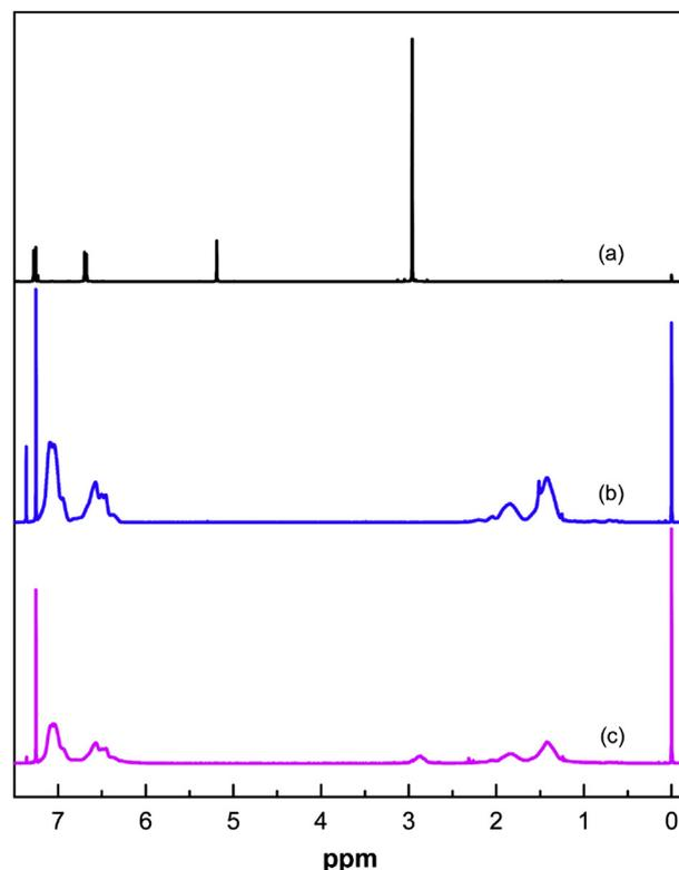
Fig. 1. <sup>1</sup>H NMR spectra (CDCl<sub>3</sub>) of BDADPE (a), polystyrene (b), and poly(styrene-co-BDADPE) (c).
