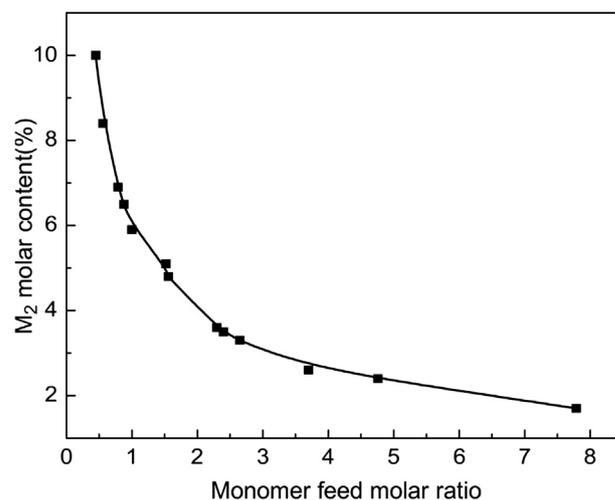
**Fig. 3.** Molar content of geminal dimethylamino groups in styrene-co-BDADPE copolymers as a function of the monomer feed molar ratio of styrene to BDADPE.
