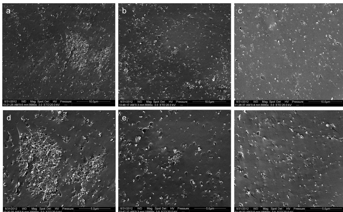
Fig. 5. SEM micrographs of fracture surface of in-chain multi-functionalized polystyrene filled with 5.22 wt% CB and the molar content of geminal dimethylamino groups: 0 for Composite 1 (a and d), 2.6% for Composite 2 (b and e) and 8.4% for Composite 3 (c and f).
