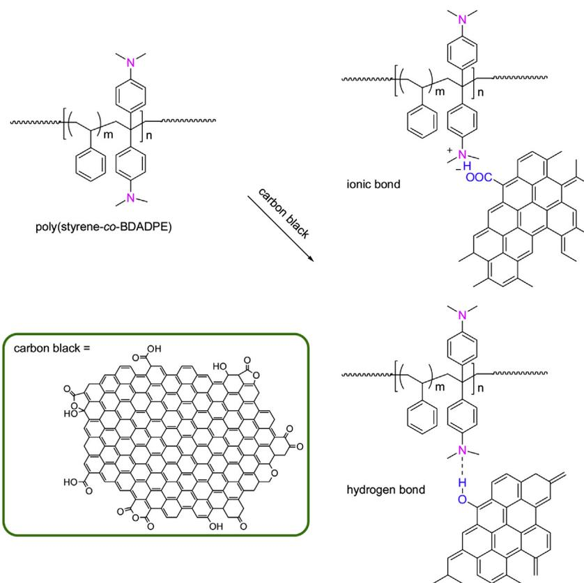
**Scheme 2.** Proposed mechanism for the formation of ionic bonds and hydrogen bonds between CB and in-chain multi-functionalized polystyrene with geminal dimethylamino groups.
