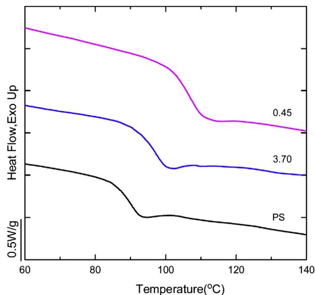
**Fig. 4.** DSC curves of poly(styrene-co-BDADPE). Each bracket indicates the corresponding monomer feed ratio.
