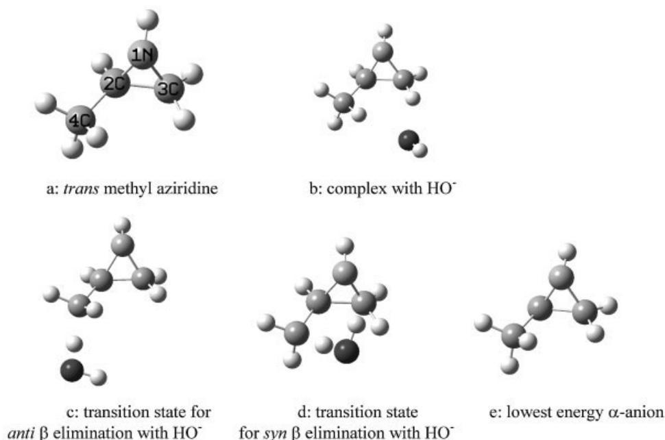
**Figure 1.** MP2/6-31+G\* optimized geometries for *trans* methyl aziridine series of compounds. (a) *trans* methyl aziridine. (b) Complex with HO<sup>-</sup>. (c) Transition state for *anti* β-elimination with HO<sup>-</sup>. (d) Transition state for *syn* β elimination with HO<sup>-</sup>. (e) Lowest energy α-anion.
