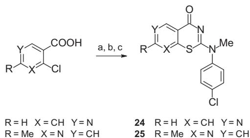
**Scheme 3.** Reagents and conditions: (a)  $\text{SOCl}_2$ , cat. DMF; (b)  $\text{NH}_4\text{SCN}$ , acetone; (c) 4-chloro-N-methylaniline, acetone.
