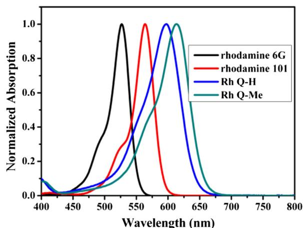
Fig. 1. The normalized UV–Vis absorption spectra of Rh Q-H, Rh Q-Me, rhodamine 101 and rhodamine 6G (ca.  $10^{-5}$  mol/L) in EtOH.
