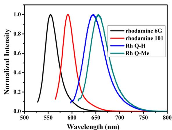
Fig. 2. The normalized fluorescence emission spectra of Rh Q-H, Rh Q-Me, rhodamine 101 and rhodamine 6G (ca.  $10^{-5}$  mol/L) in EtOH excited with 597 nm, 613 nm, 594 nm, 527 nm respectively.
