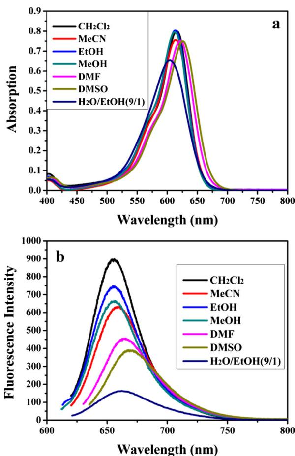
Fig. 4. UV-vis absorption (a) and fluorescence emission spectra (b) of Rh Q-Me (ca.  $10^{-5}$  mol/L) in different solvents.
