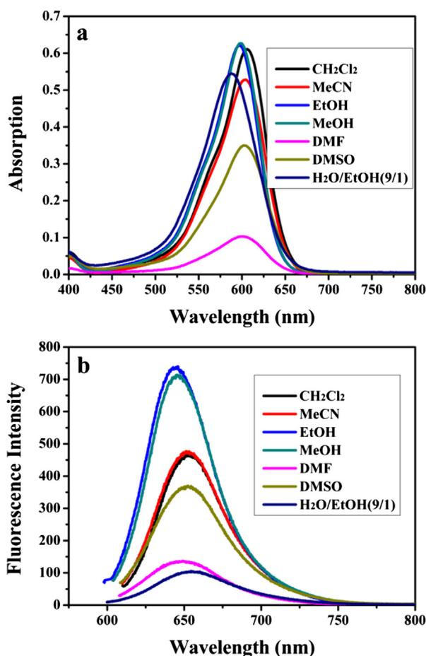
Fig. 3. UV-vis absorption (a) and fluorescence emission spectra (b) of Rh Q-H (ca.  $10^{-5}$  mol/L) in different solvents.
