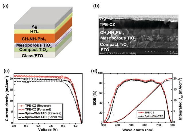
**Fig. 3** (a) Schematic of the device structure. (b) SEM cross-section image of the prepared PeSCs. (c)  $J$ - $V$  characteristics of the optimized PeSCs based on TPE-CZ as the HTL. The device based on Spiro-OMeTAD as the HTL is used for comparison. (d) The corresponding EQE spectra for the PeSCs.
