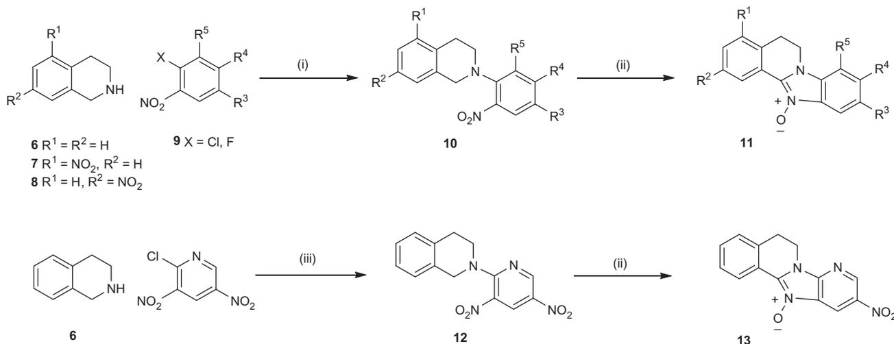
**Scheme 1.** Synthesis of nitro-substituted 5,6-dihydrobenzimidazole *N*-oxides and related derivatives. Reagents and conditions: (i) see Table 1; (ii) propionic acid, reflux; (iii) EtOH/H<sub>2</sub>O, NaHCO<sub>3</sub>, 50–60 °C.
