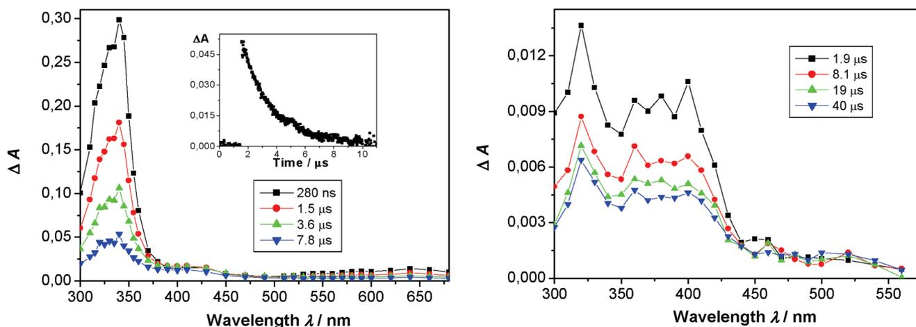
**Fig. 1** Transient absorption spectra of **1** in  $N_2$ -purged  $CH_3CN$  (left), and  $N_2$ -purged  $CH_3CN-H_2O$  (1 : 1) in the presence of  $K_2CO_3$  (right). Inset: decay at 340 nm in  $CH_3CN$ .
