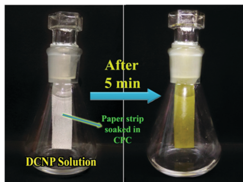
Fig. 11 Vapour phase detection of DCNP by CPC.
