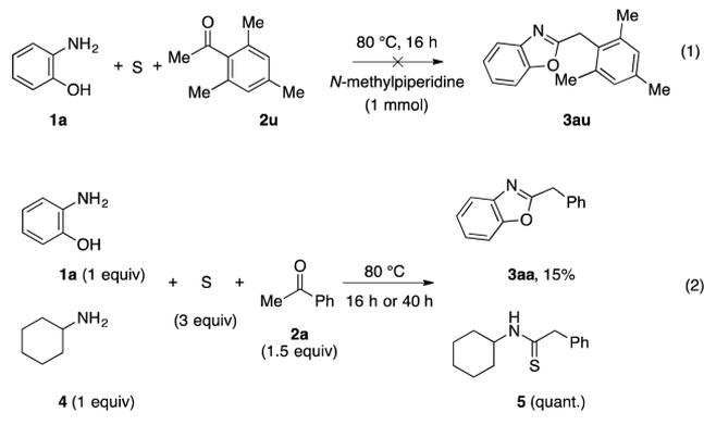
At first, in support of our working hypothesis that an attack at the carbonyl of acetophenone would initiate, we chose mesityl methyl ketone **2u** in which the carbonyl function was shielded by both *o*-methyl groups (Scheme 5, eq 1). The reaction of **2u** with **1a** did not lead to the desired benzoxazole **3au**, and starting material as well as *N*-methylpiperidine remained unchanged. This excludes the enolate species as intermediates, which are less sterically demanding.
