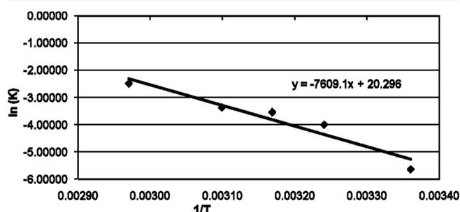
**Figure 5.** Rate data for the reaction of GB with phosphate at five temperatures, using the natural log of the rate constant of loss of GB at a concentration of 0.0307 M phosphate (with 0.1 M acetate buffer) versus reciprocal absolute temperature.
