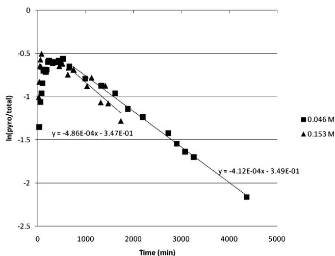
**Figure 10.** Semilog plot of the first-order rates of **1** reaction versus time for two concentrations of phosphate. The half-lives, calculated from the slope of the line for times after 500 min when the product is no longer forming, are 28.0 h for 0.046 M solution and 23.8 h for 0.153 M solution. Kinetic modeling of the data is given in the Supporting Information.
