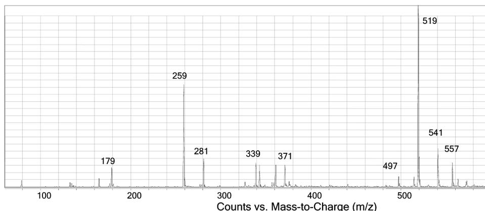
**Figure 8.** LC/MS of **2** using negative ion electrospray ionization. The  $[M-H]^-$  peak for the compound is at  $m/z$  259, and the  $m/z$  519 peak is the  $[2M-H]^-$  peak. It is interesting to observe alkali metal adducts at  $m/z$  281 for  $[M+Na-2H]^-$ ,  $m/z$  541 for  $[2M+Na-2H]^-$ , and  $m/z$  557 is  $[2M+K-2H]^-$ .
