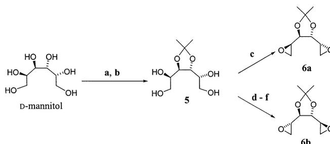
Scheme 2. (a) 2,2-DMP, pTsOH, 95%; (b) 1:10 MeOH/H<sub>2</sub>O, pTsOH, 75%; (c) (i) MeC(OMe)<sub>3</sub>, PPTS, DCM; (ii) Et<sub>3</sub>N, AcBr, DCM; (iii) K<sub>2</sub>CO<sub>3</sub>, MeOH, 95%. (d) BzCl, pyr, DCM, 72%; (e) TsCl, pyr, 100%; (f) K<sub>2</sub>CO<sub>3</sub>, MeOH, DCM, 85%.
