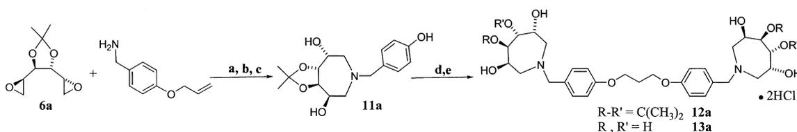
**Scheme 4.** (a) H<sub>2</sub>O, 60 °C, 69%; (b) *t*-BuOK, DMSO 100 °C, 81%; (c) HgO, HgCl<sub>2</sub> in 10:1 acetone/water, 87%; (d) K<sub>2</sub>CO<sub>3</sub>, Br(CH<sub>2</sub>)<sub>3</sub>Br, EtOH, reflux for 4 days, 31%; (e) 0.5 M HCl, 100%.
