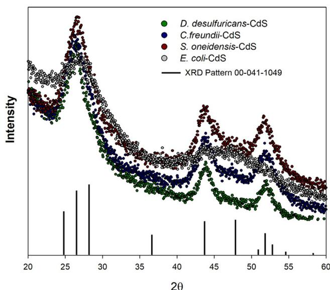
Figure 3. X-Ray diffraction patterns of the CdS biohybrid systems.
