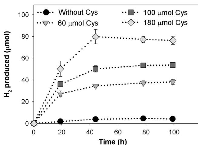
**Figure 8.** Effect of cysteine on light-driven  $H_2$  production by the *D. desulfuricans*-CdS biohybrid system. The biohybrid system was constructed under the best conditions (3 mM cadmium and 5.3 mg<sub>dw</sub>) and irradiated with LED light. The assays were carried out with 6.5 mL of working volume in the presence of MV. Error bars indicate the standard deviations of three independent experiments.
