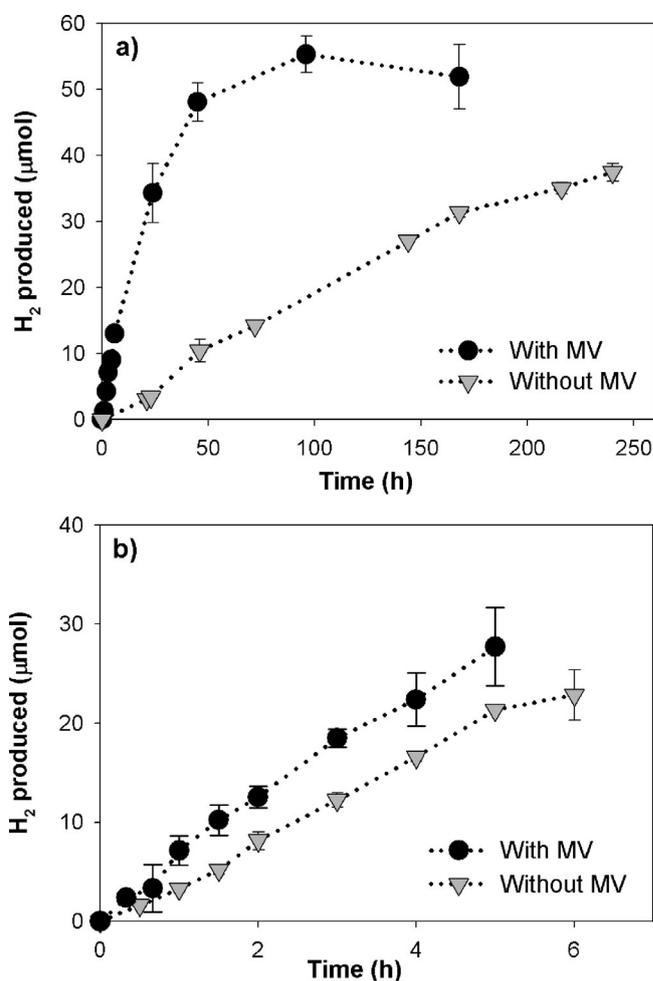
**Figure 7.** Light-driven H<sub>2</sub> production by the *D. desulfuricans*-CdS biohybrid system under two light sources: LED (a) and Xenon lamp (b), and 100 μmoles of cysteine. The biohybrid system was generated under the best conditions (3 mM cadmium and 5.3 mg<sub>dcw</sub>). The experiments were carried out with 6.5 mL of working volume. Error bars indicate the standard deviations of three independent experiments.
