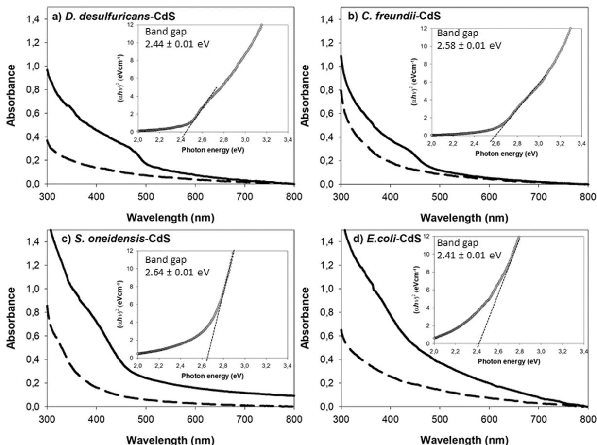
Figure 4. UV/Vis absorption spectra and Tauc Plots (inserts) of the CdS biohybrid systems. Solid and dashed lines represent the cells-CdS and cells spectra, respectively.
