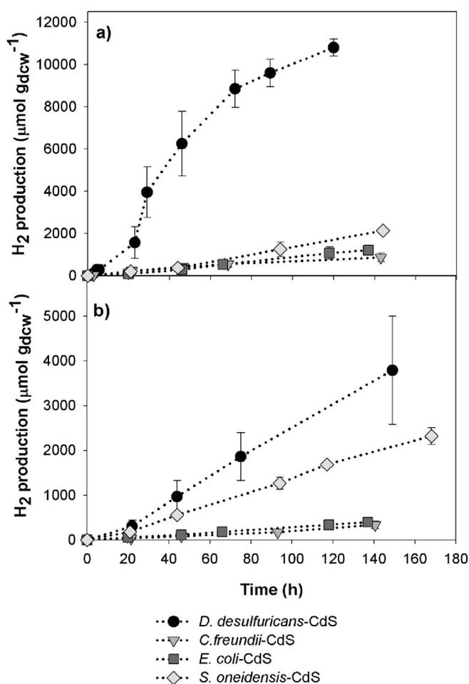
**Figure 5.** Hydrogen production profile of biohybrid systems in the presence (a) and absence (b) of methyl viologen (MV) as redox mediator. All systems were generated using 1 mM Cd. Error bars indicate the standard deviations of three independent experiments.
