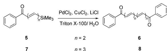
Scheme 3. Homocoupling reactions of keto-polyenylsilanes **5** and **7** in the presence of Triton X-100.
