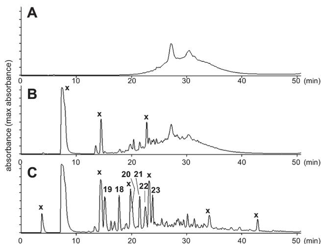
Figure 5. HPLC of the active fraction 2217 (A), the thiol degradation products of the active fraction under common reaction conditions (B), and the thiol degradation products under modified reaction conditions (C) (18–23: see Figure 6, × indicates peaks also observed in the blank).
