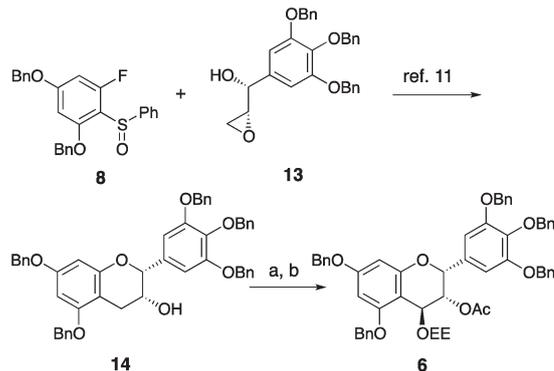
Scheme 2 Epigallocatechin unit **6**; (a) 2-ethoxyethanol, DDQ, toluene, room temp., 12 h; (b) Ac<sub>2</sub>O, DMAP, pyridine, CH<sub>2</sub>Cl<sub>2</sub>, room temp., 12 h (62%, 2 steps).
