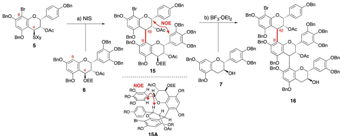
**Scheme 3** Downward assembly (a) molar ratio: **5/6/NIS** = 1.0 : 1.5 : 1.3, MS4A,  $\text{CH}_2\text{Cl}_2$ ,  $-78 \rightarrow 0$  °C over 25 min, then 0 °C, 11 h (91%); (b) molar ratio: **15/7/BF<sub>3</sub>·OEt<sub>2</sub>** = 1.0 : 1.3 : 1.9,  $\text{CH}_2\text{Cl}_2$ ,  $-78 \rightarrow -30$  °C over 1.3 h (92%).
