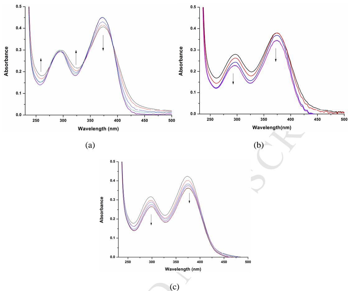
**Figure S7:** absorption spectra of probe (10  $\mu\text{M}$ ) with 200  $\mu\text{M}$  GSH (a), Hcy (b), Cys (c) in HEPES buffer (10 mM, pH 7.4,).
