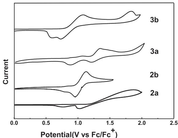
Fig. 3. Oxidation part of the CV curves of the four compounds in  $\text{CH}_2\text{Cl}_2$  solution.
