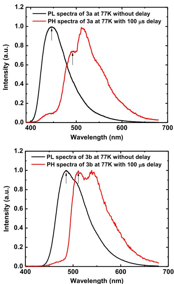
Fig. 8. The time-resolved photoluminescence (PL) and phosphorescence (PH) spectra of **3a** and **3b** in solid films with 100  $\mu$ s delay at 77 K.
