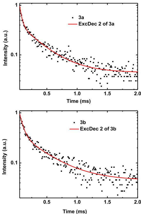
**Fig. 7.** Emission decay curves and fitting curves of **3a** and **3b** in an oxygen free atmosphere (by bubbling nitrogen through the solution for 10 min to exclude oxygen) in toluene at 300 K. The value of Adj. R-Square (>0.97) is used to ensure the quality of the fit.
