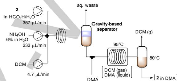
**Figure 3.** Schematic view of the continuous flow setup for the liquid-liquid extraction, phase separation and DCM-DMA solvent exchange.
