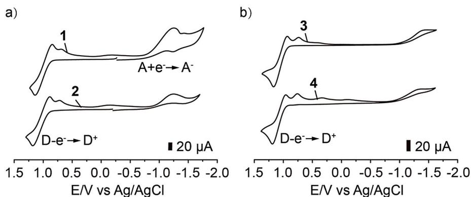
**Fig. 5.** a) Cyclic voltammograms of dyes 1 and 2,  $c = 0.005$  M; b) Cyclic voltammograms of dyes 3 and 4,  $c = 0.005$  M. Solvent: dichloromethane (0.1 M Bu<sub>4</sub>NBF<sub>6</sub>), Scanning rate: 100 mV s<sup>-1</sup> (25 °C).
