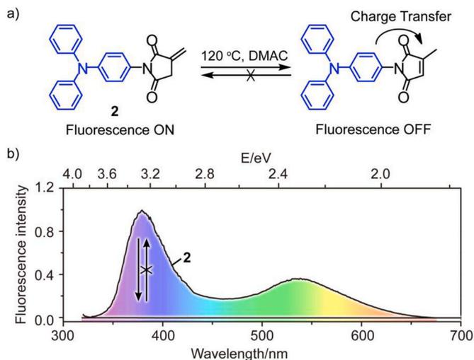
Fig. 7. Irreversible emission ON/OFF behaviours for isomerization of dye **2**. a) Isomerization of dye **2**. Reagents and conditions: *N,N*-dimethyl acetamide (DMAC),  $120$  °C, 3h. b) Fluorescence spectra in dichloromethane before and after isomerization of dye **2** in 1, 2-dichloroethane,  $[2] = 5 \times 10^{-5}$  M,  $\lambda_{\text{ex}} = 310$  nm.
