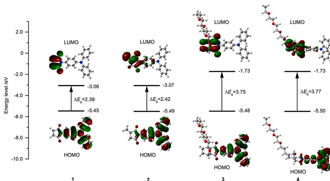
Fig. 6. Energy levels of HOMO and LUMO, energy gaps ( $\Delta E_g$ ), and electron cloud distribution of dyes 1–4 obtained by electrochemical CV measurements.
