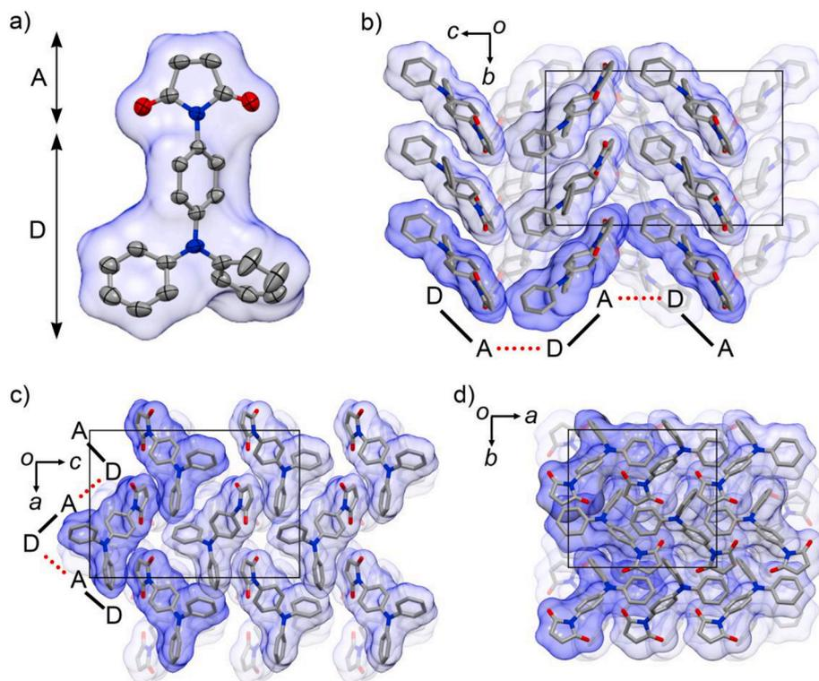
**Fig. 4.** a) Molecular structure (ORTEP) of dye 1 determined by single crystal X-ray diffraction. Thermal ellipsoids are drawn at 50% probability level. Crystal packing diagrams of dye 1 along the *a*-axis (b), along the *b*-axis (c) and along the *c*-axis (d). Intermolecular donor-acceptor dipole interactions are indicated by red dotted lines in (b) and (c). (For interpretation of the references to colour in this figure legend, the reader is referred to the Web version of this article.)
