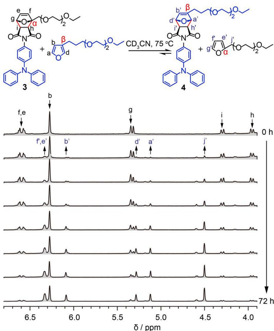
**Fig. 9.** Dynamic furan moiety exchanges during the conversion of  $\alpha$ -position furan-substituted dye **3** into  $\beta$ -position dye **4** monitored by  $^1\text{H}$  NMR spectroscopy.  $[\mathbf{3}] = 0.05\text{ M}$ . Reaction time are 0, 3, 6, 12, 24, 36, 48 and 72 h from top to bottom, respectively.
