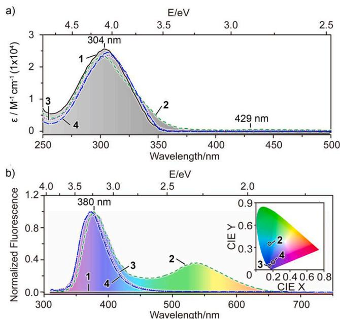
**Fig. 3.** a) UV-vis absorption spectra of dyes 1–4 in 1, 2-dichloroethane,  $c = 5 \times 10^{-5}$  M; b) Fluorescence spectra of dyes 1–4 in 1, 2-dichloroethane,  $c = 5 \times 10^{-5}$  M,  $\lambda_{\text{ex}} = 310$  nm. Inset: CIE 1931 chromaticity diagram, three points are emission colour coordinates of 2 (0.16, 0.34), 3 (0.16, 0.06), 4 (0.20, 0.10)). (For interpretation of the references to colour in this figure legend, the reader is referred to the Web version of this article.)
