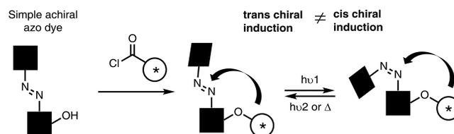
Figure 1. Concept of converting an industrial dye to a light-triggered chiroptical switch.
