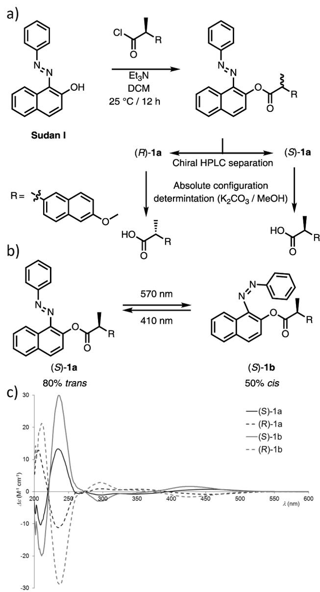
Scheme 1. a) Synthesis, resolution and determination of absolute configuration of **1a**; b) photoisomerization of (*S*)-**1a** to (*S*)-**1b**; c) CD spectra of (*S*)- and (*R*)-**1a–b** in solution in acetonitrile ( $c = 6 \times 10^{-6}$  M).
