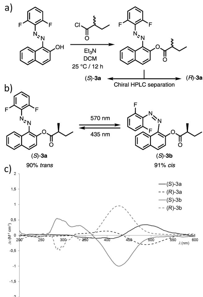
Scheme 3. a) Synthesis and resolution of **3a**; b) photoisomerization of (*S*)-**3a** to (*S*)-**3b**; c) CD spectra of (*S*)- and (*R*)-*trans*-**3a** and (*S*)- and (*R*)-*cis*-**3b** in acetonitrile ( $c = 6 \times 10^{-5}$  M).
