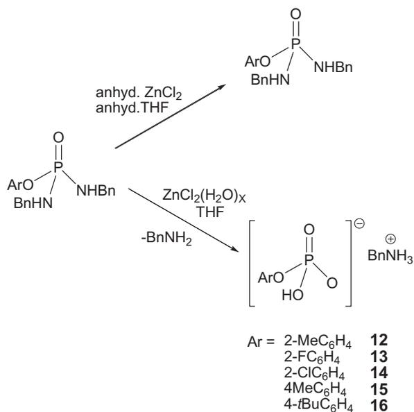
Scheme 3. Reaction of  $N,N'$ -dibenzylphosphorodiamidate with  $\text{ZnCl}_2$ .
