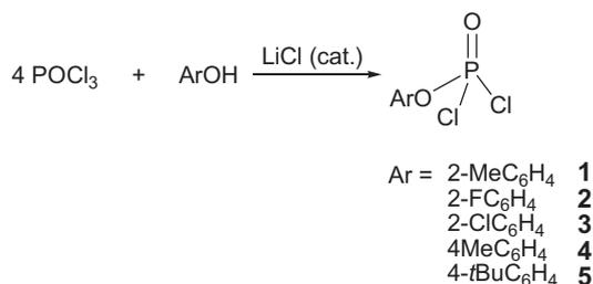
**Scheme 1.** Synthesis of phosphodichloridates.
