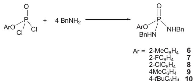
**Scheme 2.** Synthesis of *N,N'*-dibenzylphosphorodiamidate.
