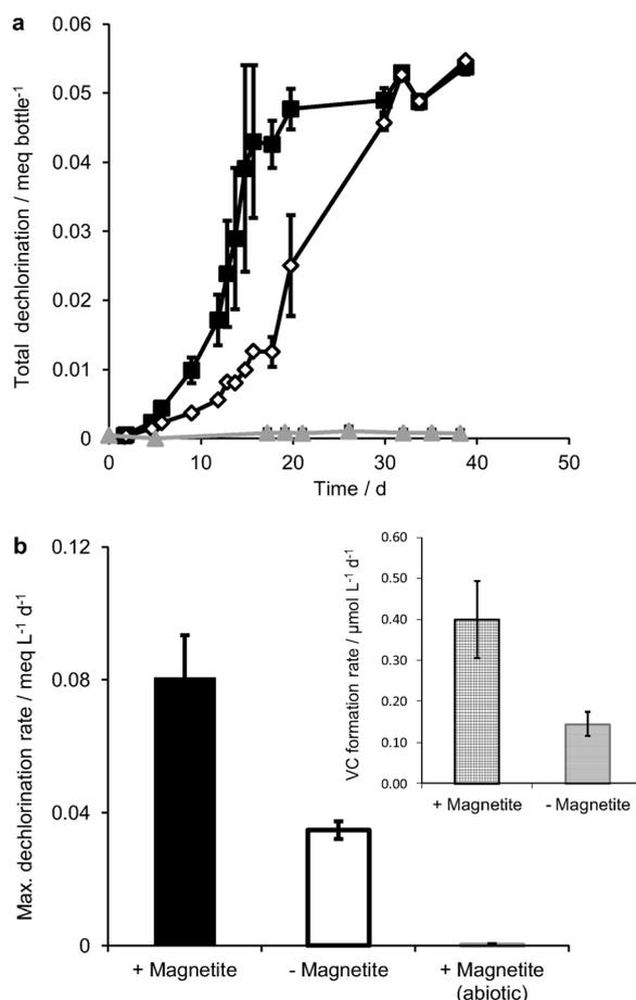
**Figure 2.** a) Cumulative respiratory electrons channeled to TCE dechlorination, and b) maximum rates of TCE dechlorination for the batch experiments depicted in Figure 1. The effect of magnetite nanoparticles on the maximum rate of VC formation is highlighted as an insert in (b). Error bars (when larger than symbols) represent  $\pm 1$  standard deviation of replicated experiments.  $\blacksquare$ : + magnetite,  $\diamond$ : - magnetite,  $\blacktriangle$ : + magnetite (abiotic).
