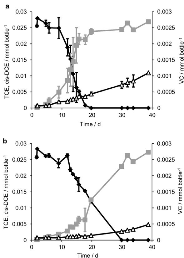
**Figure 1.** Time course of TCE dechlorination with acetate ( $20 \text{ mmol L}^{-1}$ ) as electron donor in anaerobic serum bottles a) supplemented, or b) not supplemented with conductive magnetite nanoparticles. Error bars (when larger than symbols) represent  $\pm 1$  standard deviation of replicated experiments.  $\blacklozenge$ : TCE,  $\blacksquare$ : cis-DCE,  $\blacktriangle$ : VC.
