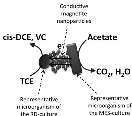
**Figure 4.** Conceptual illustration of the proposed interspecies electron transfer between dechlorinating and non-dechlorinating microorganisms, through conductive magnetite nanoparticles.
