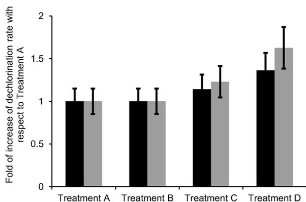
**Figure 3.** Effect of magnetite nanoparticles and the MES-culture on the maximum rate of TCE dechlorination by the RD-culture, in the presence of acetate ( $20 \text{ mmol L}^{-1}$ ). Error bars (when larger than symbols) represent  $\pm 1$  standard deviation of replicated experiments. Treatment A: RD-culture, treatment B: RD-culture + magnetite, treatment C: RD-culture + MES-culture, treatment D: RD-culture + MES-culture + magnetite. ■: 1st feeding cycle, ■: 2nd feeding cycle.
