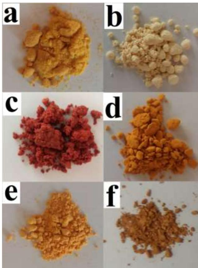
**Figure 5.** Synthesized powder of the frameworks and related N-donor ligands. (a) BPDB pillar spacer for construction of TMU-4. (b) As-synthesized powder of TMU-4. (c) H<sub>2</sub>DPT pillar spacer for construction of TMU-34. (d) As-synthesized powder of TMU-34. (e) As-synthesized powder of SALE-TMU-34. (f) As-synthesized powder of USALE-TMU-34.
