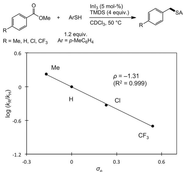
Figure 2. Hammett plot for the  $\text{InI}_3$ -catalyzed reductive sulfidation of the *p*-substituted methyl benzoates *p*-RC<sub>6</sub>H<sub>4</sub>CO<sub>2</sub>Me (R = Me, H, Cl, CF<sub>3</sub>).
