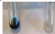
Figure 3. Reaction tubes containing KOTBu and 17 in benzene (a) left: exposed to 400 nm light and (b) right: shielded from light by covering in foil.
