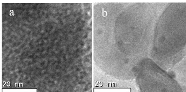
**Fig. 1** HRTEM images of supported gold catalysts: (a) 1.0 wt% Au/Fe(OH)<sub>x</sub>, (b) 1.1 wt% Au/Fe<sub>2</sub>O<sub>3</sub>-4.
