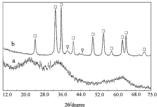
**Fig. 2** X-Ray diffraction patterns for supported Au catalysts: (a) 1.0 wt% Au/Fe(OH)<sub>x</sub>, (b) 1.1 wt% Au/Fe<sub>2</sub>O<sub>3</sub>-4. (□) hematite; (▽) metallic gold.
