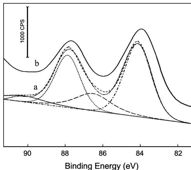
**Fig. 3** XPS spectra of supported Au catalysts: (a) 1.0 wt% Au/Fe(OH)<sub>x</sub>, (b) 1.1 wt% Au/Fe<sub>2</sub>O<sub>3</sub>-4.
