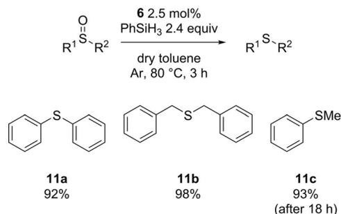
**Scheme 2.** Borinic acid catalyzed reduction of sulfoxides.
