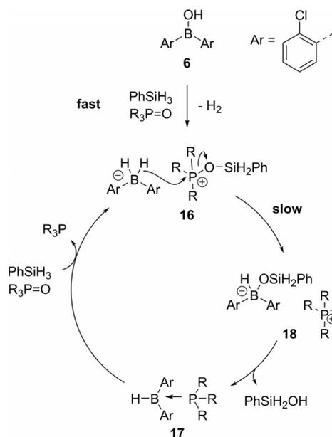
Scheme 5. Mechanism of the reduction.
