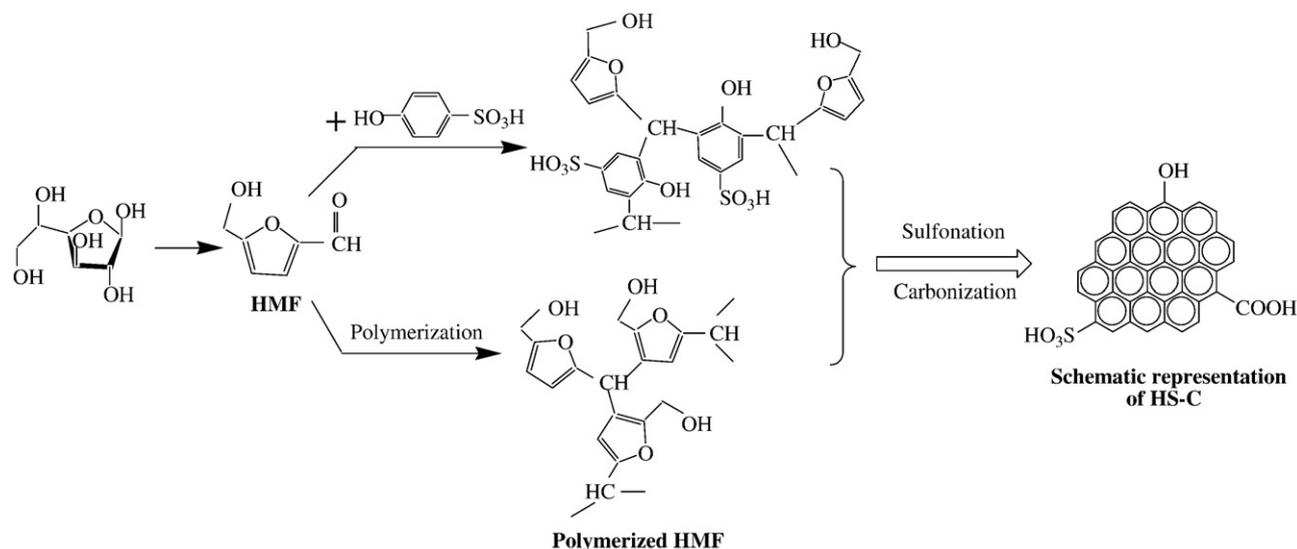
Fig. 1. Schematic diagram for the synthesis of acidic carbon materials from glucose and 4-hydroxybenzenesulfonic acid.
