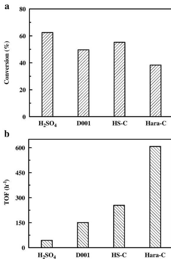
Fig. 5. Conversion of isopentene and rate of formation of TAME (TOF) for the reaction of isopentene with methanol at 353 K after 20 h.
