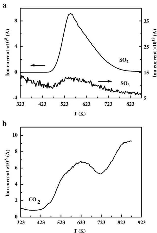
Fig. 4. Evolution of SO<sub>2</sub>, SO<sub>3</sub> and CO<sub>2</sub> from HS-C when it was linearly heated in N<sub>2</sub> during the TG-MS measurement.
