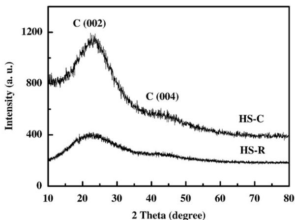
Fig. 2. X-ray diffraction patterns of HS-R and HS-C.
