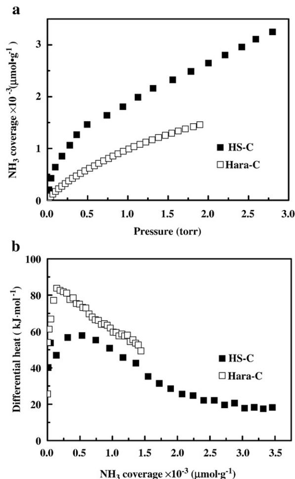
Fig. 3. Microcalorimetric adsorption of NH<sub>3</sub> at 353 K over HS-C and Hara-C.
