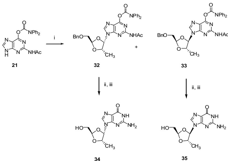
**Scheme 5.** Reagents and conditions: (i) a. bis-(trimethylsilyl)acetamide, 1,2-dichloroethane, b. **20**, trimethylsilyl triflate, reflux; (ii) hydrazine hydrate, tetrahydrofuran, reflux; (iii) palladium hydroxide/C, ethanol, cyclohexene.
