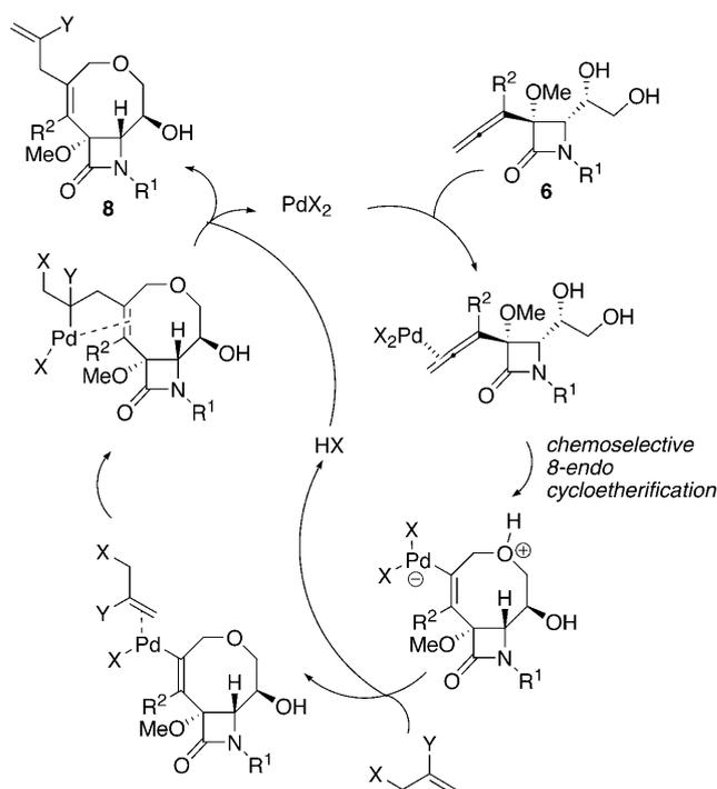
Scheme 6. Mechanistic explanation for the Pd<sup>II</sup>-catalyzed heterocyclizative coupling reaction of  $\gamma,\delta$ -allendiols **6**.
