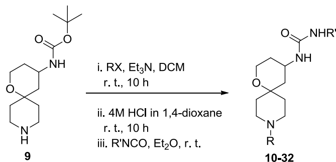
Scheme 2. Synthesis of spirocyclic sEH inhibitors based on core building block 9 .
