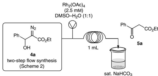
**Scheme 3** Flow set-up for the three-step process
