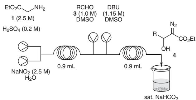
**Scheme 2** Continuous flow setup for the two-step process
