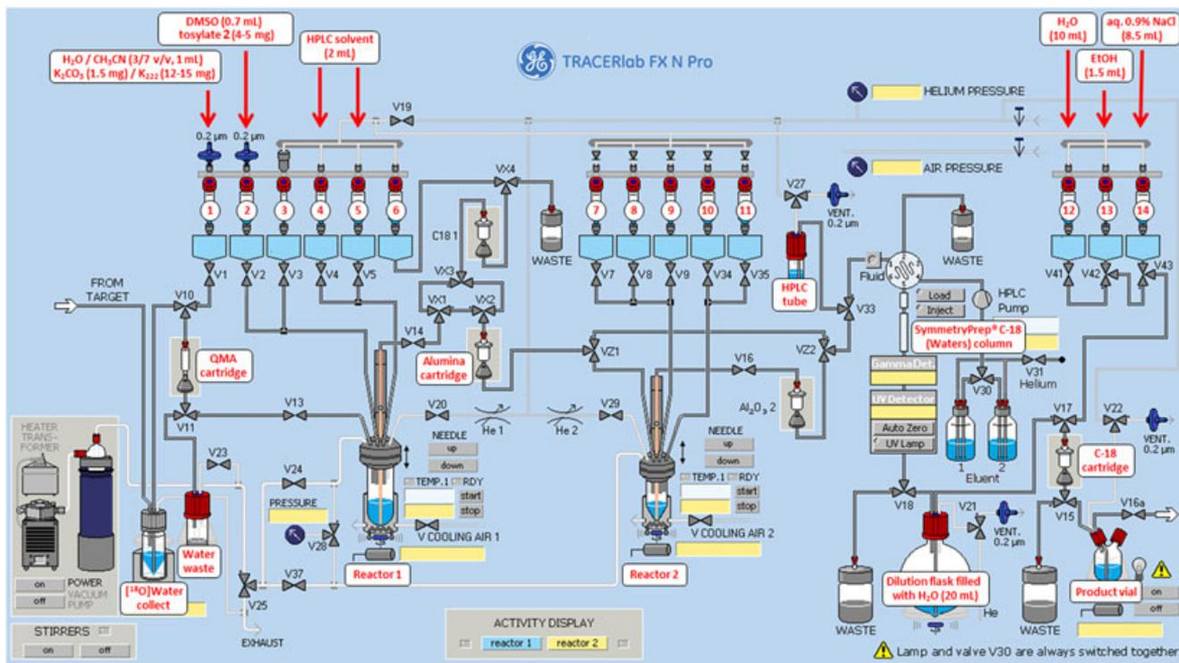
**Figure 2.** Description of the TRACERlab FX N Pro synthesizer used for the preparation of [<sup>18</sup>F]DPA-C5yne ([<sup>18</sup>F]-1) and positioning of all required reagents, solvents and consumables.
