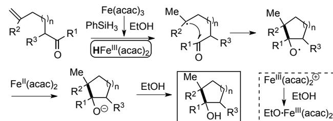
**Scheme 3.** Overview of the proposed reaction mechanism.
