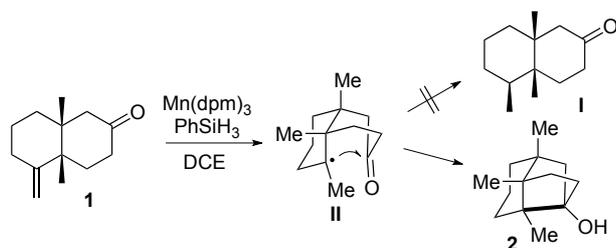
**Scheme 2.** Intramolecular coupling vs reduction under HAT reaction conditions.
