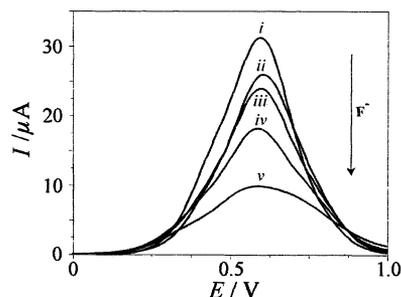
Fig. 7. DPV of a poly(VTPAB<sub>2</sub>) film (electropolymerisation charge, 150 mC cm<sup>-2</sup>) in CH<sub>3</sub>CN + 0.1 M Bu<sub>4</sub>NClO<sub>4</sub> without (i) and with 0.1 mM (ii), 0.5 mM (iii), 1.0 mM (iv) and 2.0 mM (v) of Et<sub>3</sub>N·3 HF.
