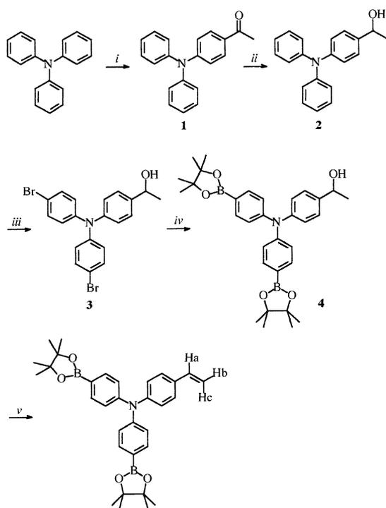
Scheme 1. Synthesis of the vinyl-substituted bipodal redox-active receptor **VTPAB<sub>2</sub>**. Reagents and conditions: (i) acetic anhydride, toluene, then addition of  $SnCl_4$ , reflux, 1 h. [9]; (ii)  $LiAlH_4$ , anhydrous THF,  $0^\circ C$ ; (iii)  $Br_2$ ,  $CHCl_3$ ,  $-20^\circ C$ ; (iv)  $n-BuLi$ , trimethyl borate, anhydrous diethyl ether,  $-78^\circ C$ , pinacol,  $25^\circ C$ ; (v)  $POCl_3$ , pyridine, reflux,  $> 12$  h.
