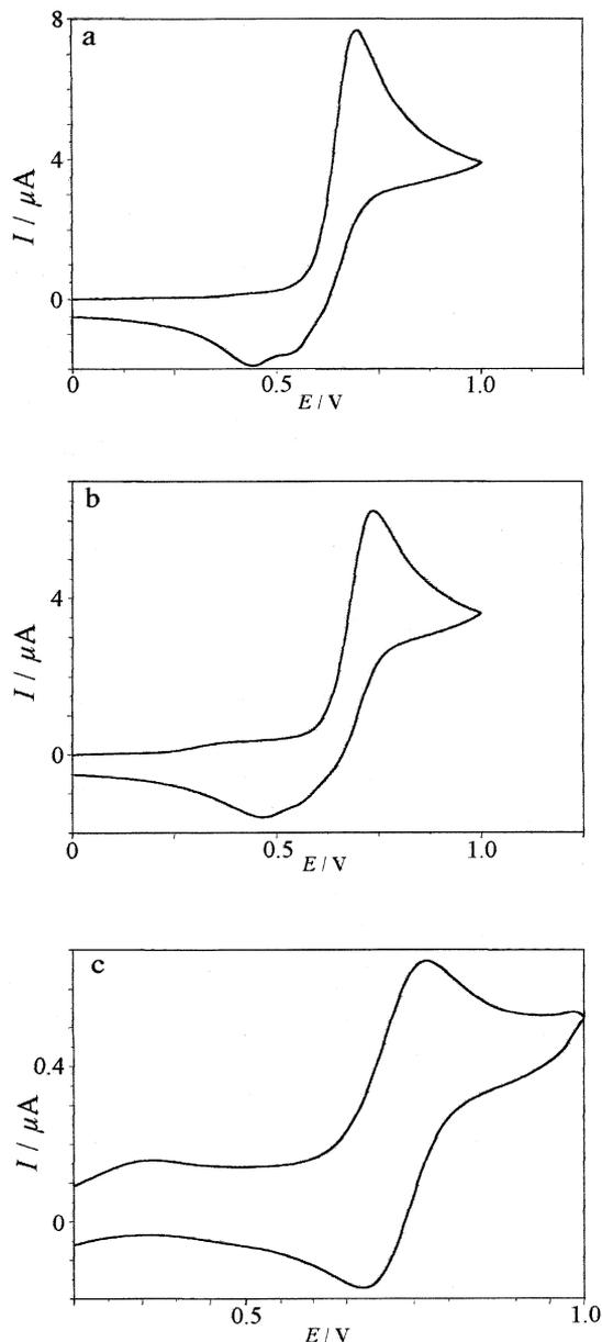
Fig. 2. Cyclic voltammograms in  $\text{CH}_3\text{CN} + 0.1 \text{ M Bu}_4\text{NClO}_4$  of: (a) **TPAB<sub>1</sub>** (2 mM); (b) **TPAB<sub>2</sub>** (2 mM); and (c) **TPAB<sub>3</sub>** (1.5 mM). Potential scan rate:  $0.1 \text{ V s}^{-1}$ .
