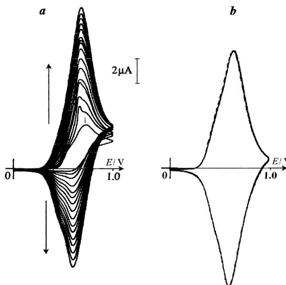
Fig. 6. (a) Potentiodynamical electropolymerisation of VTPAB<sub>2</sub> at 5 mM in  $CH_3CN + 0.1$  M  $Bu_4NClO_4$  and (b) response of the resulting polymer film in the same electrolytic solution; first cycle (—) and tenth cycle (— —). Potential scan rate: 50  $mV s^{-1}$ .
