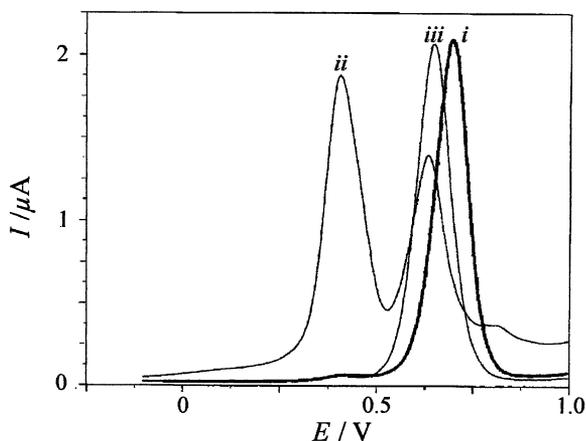
Fig. 5. DPV in  $CH_2Cl_2 + 0.1$  M  $Bu_4NClO_4$  of TPAB<sub>1</sub> (1 mM) before (i) and after addition of 5 mM  $Et_3N \cdot 3 HF$  (ii) and then 10 mM  $Me_3SiCl$  (iii).
