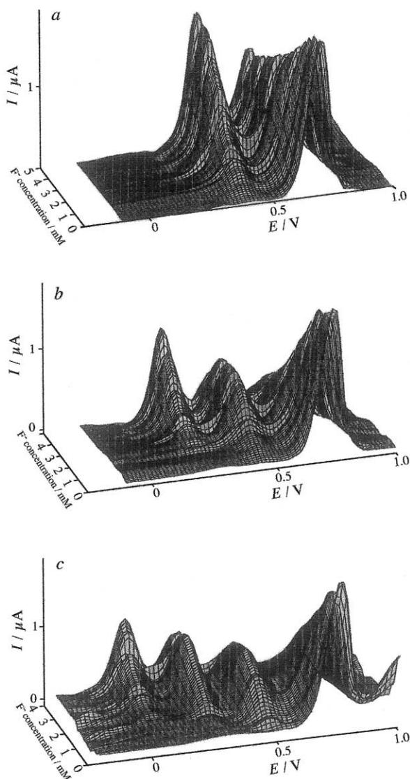
Fig. 4. Three-dimensional view of differential pulse voltammograms DPV in  $\text{CH}_2\text{Cl}_2 + 0.1 \text{ M Bu}_4\text{NClO}_4$  of: (a)  $\text{TPAB}_1$ ; (b)  $\text{TPAB}_2$ ; and (c)  $\text{TPAB}_3$  at 1 mM, as a function of the  $\text{Et}_3\text{N} \cdot 3 \text{ HF}$  concentration (from 0 to 5 mM). DPV parameters: modulation time, 0.1 s; interval time, 1 s; modulation amplitude, 50 mV.
