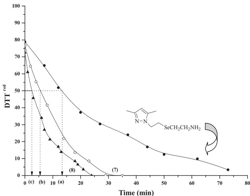
**Figure 4**  $\text{DTT}^{\text{red}} = 23.1 \text{ mg}$  (0.15 mmol),  $\text{H}_2\text{O}_2 = 9.5 \mu\text{L}$  (45.96%, 0.15 mmol), catalyst concentration =  $1.6 \mu\text{mol}$ .
