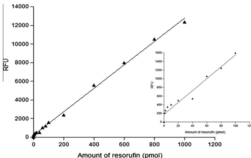
**Fig. 2.** Standard graph of resorufin. The fluorescence response due to resorufin was linear from 1 to 1000 pmol, indicating its utility in developing a sensitive optical assay for Lgt. The inset shows the useful range of 1 to 100 pmol under the assay conditions for Lgt.
