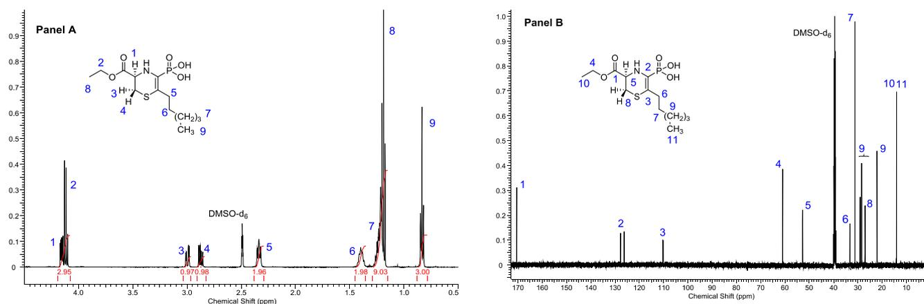
**Fig. 1.**  $^1\text{H}$  (Panel A, Left) and  $^{13}\text{C}$  (Panel B, Right) NMR spectra of 2-*n*-hexyl-LKE-P.
