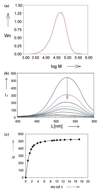
**Figure 3.** (a) Molecular weight and polydispersity determination for homopolymer 1 by GPC; (b) fluorescence spectra from titration of 1a (1  $\mu$ M) with cytochrome *c*; (c) corresponding titration curve (inverted intensity decrease).
