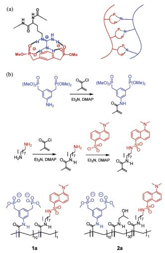
Figure 1. (a) Left: structural key element - arginine residue embraced by bisphosphonate dianion. Right: schematic depicting the multiplication of bisphosphonate units for oligoarginine recogntion. (b) Synthesis of monomer building blocks as well as schematic structure of homo- and copolymer 1a and 2a.
