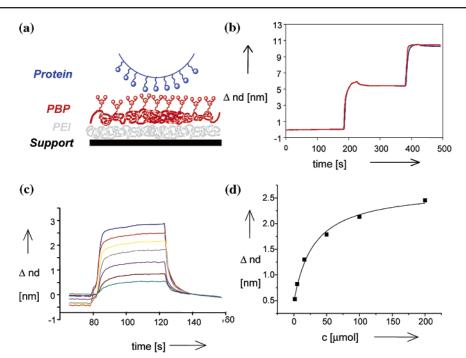
*Figure 7.* (a) Schematic showing the attachment of molecular PEI and PBP layers onto the signal transducer; (b) Corresponding stepswise increase in RIfS signal. (c) RIfS signal upon injection of trypsin at different concentrations, binding on 1 with reversible and irreversible contributions; (d) corresponding titration curve furnishing  $K_a$ .
