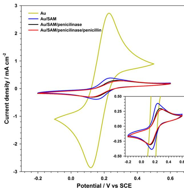
Fig. 2. Cyclic voltammeteries of a ferrocene solution, 2 mmol L<sup>-1</sup>, in KNO<sub>3</sub>, 1 mol L<sup>-1</sup>, with different electrode surfaces: bare gold; gold and cysteine SAM; gold, cysteine SAM with penicillinase; and gold, cysteine SAM with penicillinase and the analyte penicillin. Inlay: detail of lower currents.
