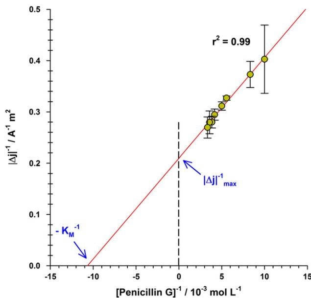
Fig. 4. Double-reciprocal plot (also known as Lineweaver–Burk plot) used to calculate the  $K_M$ .
