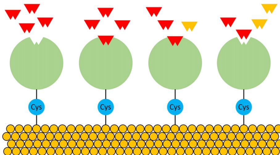
Fig. 1. Schematics of the experimental configuration, β-lactamases are connected to the gold electrode surface by cysteine molecules. Penicillin G molecules in solution react with the β-lactamases (molecules are not drawn to scale).
