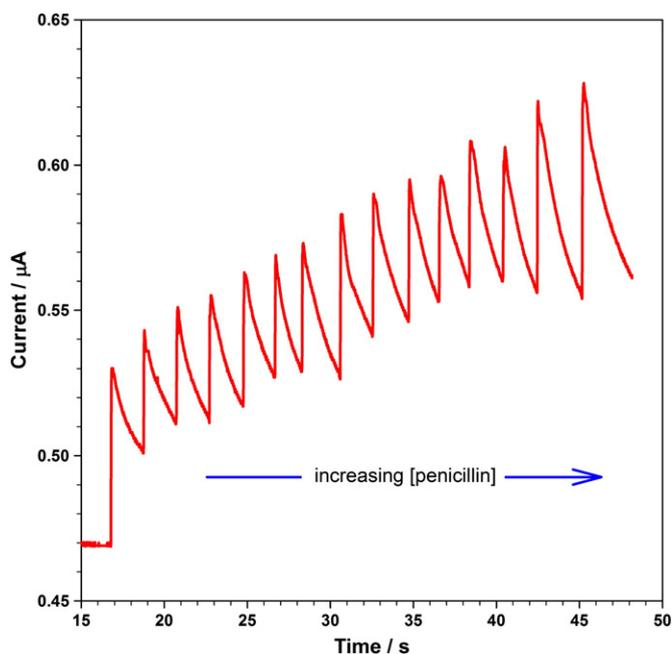
Fig. 3. Example of a chronoamperometry. Current was measured while subsequently increasing concentrations of penicillin were injected to the system (each concentration had an increment of  $20 \mu\text{mol L}^{-1}$ ).
