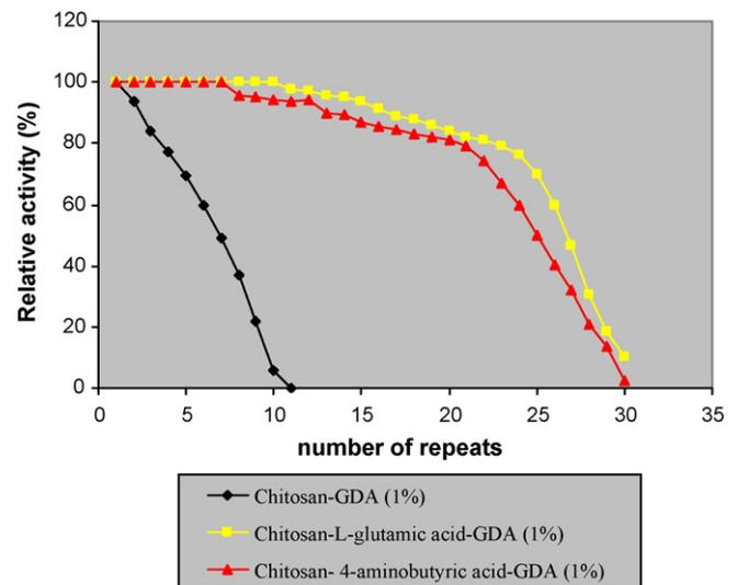
**Fig. 13.** Influence of repeats on the activities of the immobilized cellulase on chitosan-GDA (1%), chitosan-L-glutamic acid-GDA (1%) and chitosan-4-aminobutyric acid-GDA (1%), via cross-linking method.
