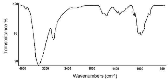
**Fig. 3.** FT-IR spectrum of chitosan–4-aminobutyric acid.
