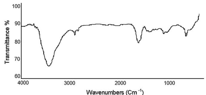
**Fig. 4.** FT-IR spectrum of chitosan–GDA (1%).
