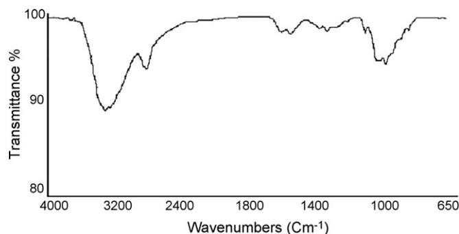
**Fig. 1.** FT-IR spectrum of chitosan.
