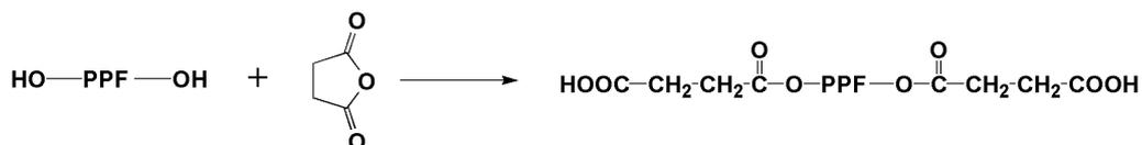
Fig. 2. Reaction between poly(propylene fumarate)-diol (PPF-diol) and succinic anhydride for the preparation of poly(propylene fumarate)-di-succinate (PPF-succinate).
