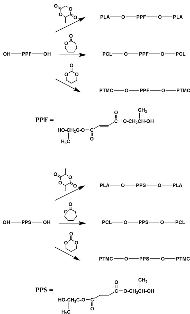
Fig. 3. Preparation of triblock copoly(propylene fumarate or succinate) with cyclic monomers.
