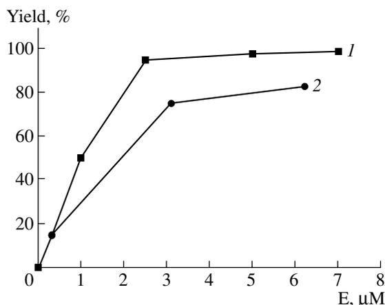
Fig. 2. The yields of Z-Ala-Ala-Leu-Phe-pNA in the syntheses catalyzed by SDS complexes of (1) subtilisin Karlsberg and (2) subtilisin 72 in ethanol. The synthetic conditions: [S] was 30 mM, 3 : 7 DMF–ethanol (vol), 0.5 h.
