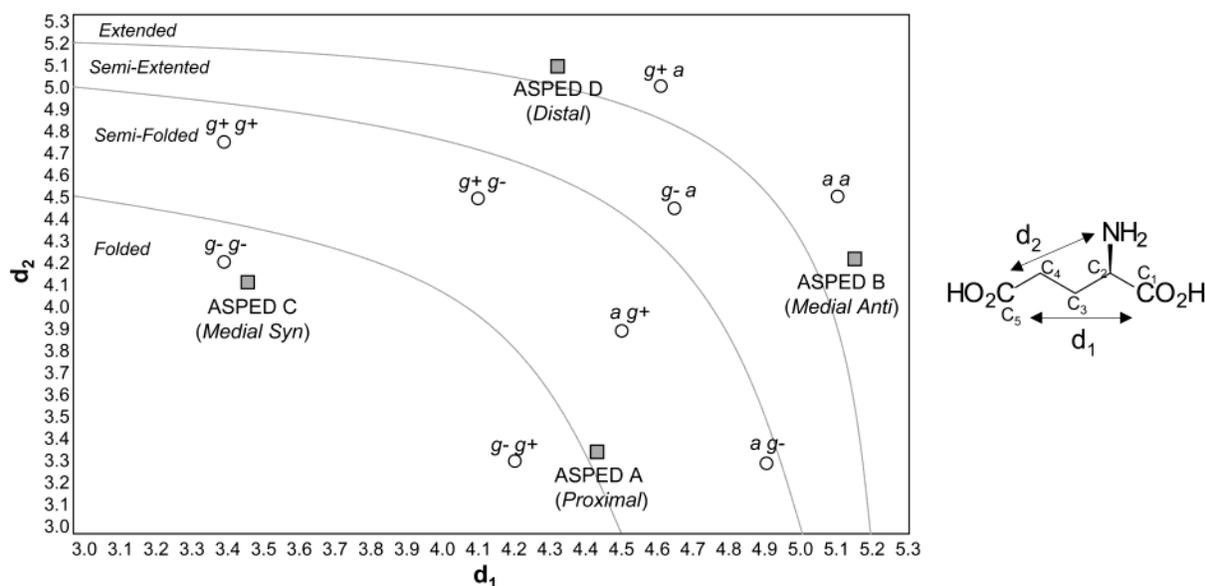
**FIGURE 1.** Projection of the four pairs of diastereoisomers of trisubstituted spiropentanes **22a–d** and of the nine staggered conformations of glutamate, into a bidimensional plot according to the  $d_1, d_2$  distances;  $d_1$  is defined as the distance between the carbons of the two carboxylate groups (C–C), and  $d_2$  is defined as the distance between the carbon of the distal carboxylate group and the nitrogen of the amino acidic amino group.
