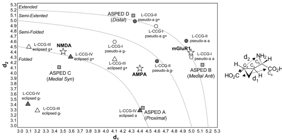
**FIGURE 2.** Comparison between **22a–d** and carboxycyclopropylglycine in the  $d_1$ – $d_2$  space. Again,  $d_1$  is defined as the distance between the carbons of carboxylate groups (C–C), and  $d_2$  is defined as the distance between the carbon of the distal carboxylate group and the nitrogen of the amino acidic amino group. Stars indicate the projection of the proposed bioactive conformations of glutamate when acting at selected iGluR's or mGluR's.
