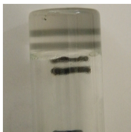
Figure 1. Typical gel formed from 0.5 wt % L in toluene with cooling in a water bath. Lines drawn on the background paper help to show the high degree of translucency in these gels. The lines behind the gel are of the same length as the two below the gel but are magnified by the curvature of the vial.
